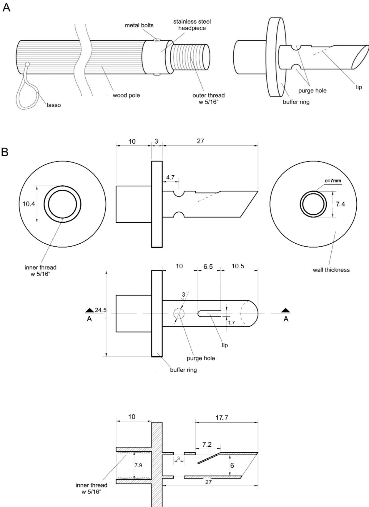
Showing (A) schematic of the biopsy pole system and detail of distal part, including biopsy tip and (B) detailed schematic of the biopsy tip.
